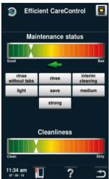
Efficient CareControl detects when the appliance needs to be cleaned. Efficient CareControl takes into account the individual cleaning behaviour and work routines such as longer breaks or the end of work.
