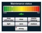
The recommended cleaning stage is highlighted in colour.
