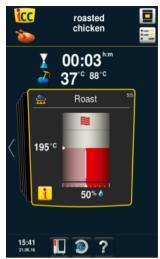
Roast in combination of steam and convection (50% humidity at 202°C cooking chamber temperature).
