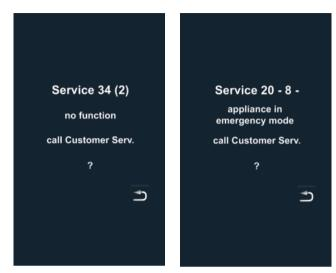
If faults occur on your unit, they are indicated on the display: Please note the phone number for fast contact with your customer service department. Faults on your unit which allow you to carry on cooking can be suppressed by pressing the "back" button.
